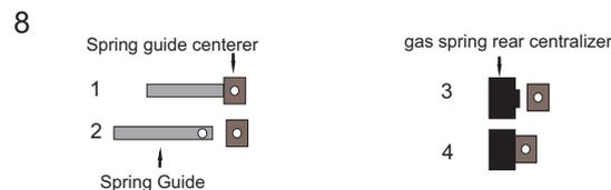
Unhook the spring guide from the centralizer. Fit the rear gas spring centerer into the spring guide centerer.
