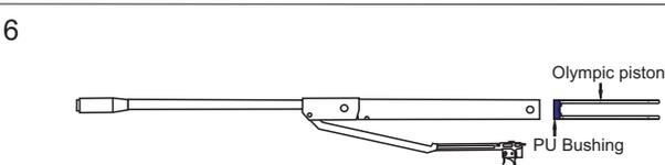
Insert the plunger by rotating the carbine cylinder to avoid cuts in the PU bushing.
