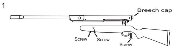
Remove the 3 screws from the stock, and remove the stock. Attach the carbine and operate a spring compressor over the breech cover.
