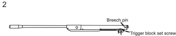
Remove the set screw from the trigger block with a spanner 10. Remove the pin that secures the breech cover and decompress the spring.
