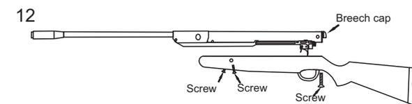
Check that the parts are all in place (lever roller and lever support). Fit the stock and tighten the 3 screws with low torque chemical lock.
