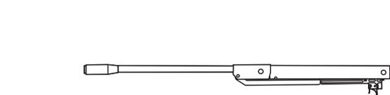
Fit the rifle's cocking lever. Install the trigger mechanism.
