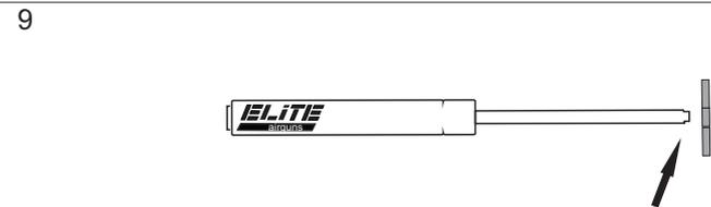
Fit the centralizer to the lowering of the Gas Ram
