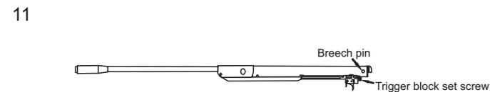
Install the pin that transfers the centralizer. Screw the trigger block's set screw using a low torque chemical lock.
