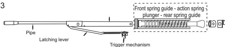
Break the barrel and detach the trigger mechanism. Unclip the cocking lever. Remove the parts that will no longer be used.
