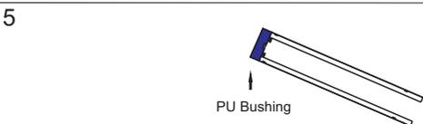
Use the silicone grease, lubricant that comes with the kit, on the side of the PU bushing. Use little lubrication, as excess lubrication causes diesel effect and damages the bushing
